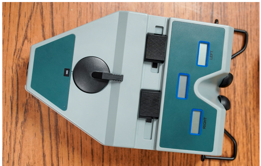
A device that the volunteers at Bart's Place use to measure the distance between the left and right pupils of a patient. These measurements are used to select the correct frame size for a new pair of glasses. || Photo by Caleb Hennington
